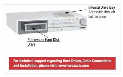
The internal drive bay is located in the bottom panel of the DVR as referenced above.
